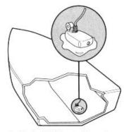
Inside the Hull Mounted Transducer
